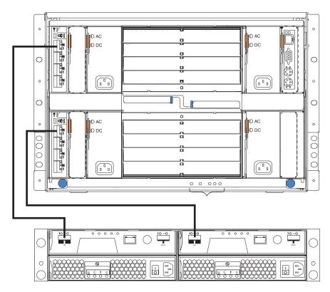
Figure 32. Example of a DS3200 that is connected to one BladeCenter unit
